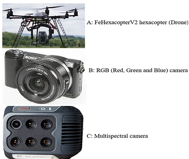
FIGURE 2 Drone (A), red, green, and blue (RGB) (B), and multispectral (C) cameras used in the image capture during the experiments in Senegal and Mali.
