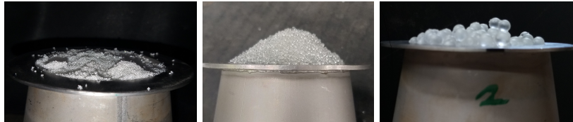
Fig. 22 Various shapes of rupture surface observed with the large macroscopic cone: (left) almost planar rupture for a sample of 0.6 mm beads with X_p = 0.5 %; (middle) roughly parabolic curved shape for a sample of 1.4 mm beads with X_p = 0.2 %; (right) moderately curved shape for a sample of 7 mm beads with X_p = 0.5 %.
