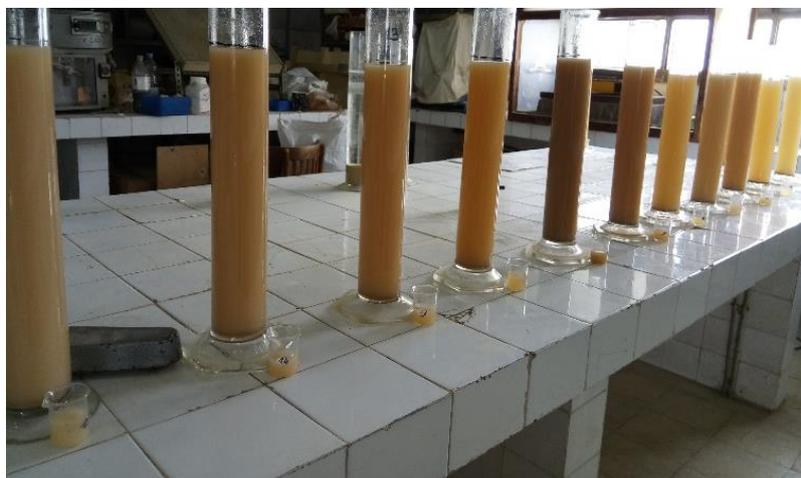
*Image 4: Sedimentation step of the granulometric test*
