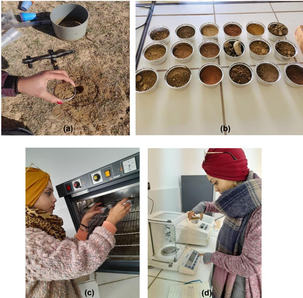
*Image 2: (a), (b), (c) and (d) illustrating steps for bulk density determination*
