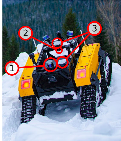
Figure 7. Experimental setup for the WILN system on our Clearpath Robotics Warthog UGV. Left: Detailed specifications. Right: The numbers in red circles correspond to (1) Robosense RS-32 lidar, (2) XSens MTi-10 IMU, and (3) two Emlid Reach-RS+ GNSS antennas. The two GNSS antennas are not used for the localization of the WILN system.
