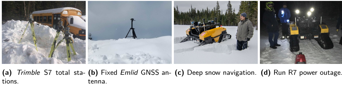
Figure 19. Various lessons learned during this deployment. (a) Total stations that were intended to measure the ground truth localization of the UGV in the Garage area. Despite considerable effort to prevent sinkage, those devices shifted significantly, resulting in unusable data. (b) The fixed GNSS antenna to enable RTK-GNSS. This device was placed in open areas to ensure good GNSS signal reception. (c) The Warthog UGV navigating in deep snow. A 1.8 m tall human operator stands next to the robot for scale. The snow level is estimated at 0.7 m in this area. The bottom of the robot chassis is resting directly on snow, affecting traction and eventually leading to UGV immobilization. (d) Warthog battery failure during run R7. A generator (in red) was used to recharge the robot batteries and later drive it manually back to the Garage POI.
