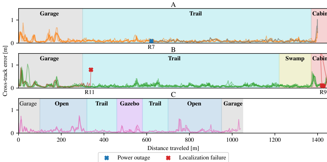
Figure 11. Cross-track error with respect to distance traveled for all runs. The results from paths A , B , and C are plotted in orange, green, and pink, respectively. The three localization failures from runs R9 and R11 are depicted as red crosses. Run R7, which ended prematurely due to a battery outage, is depicted as a blue cross. The shaded areas for each path correspond to those shown in Figure 10.
