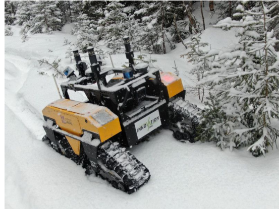
Figure 18. The result of a failed localization initialization, during run R9. The high initial error in robot pose resulted in the Warthog diverging from the reference path and heading towards vegetation. The robot reached a 2.25 m deviation before being manually stopped and driven back to the initialization position.
