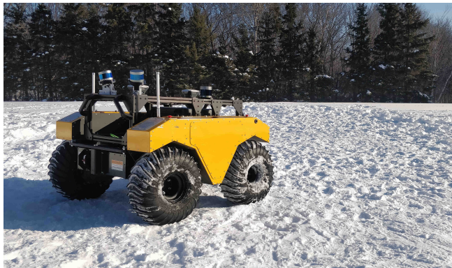
Figure 1: The wheeled skid-steer platform, a Warthog from Clearpath , on a snow-covered testing site. Due to the steering type and the snow on the ground, the robot is very prone to skidding and slippage, making the control and state estimation of this system quite challenging.
