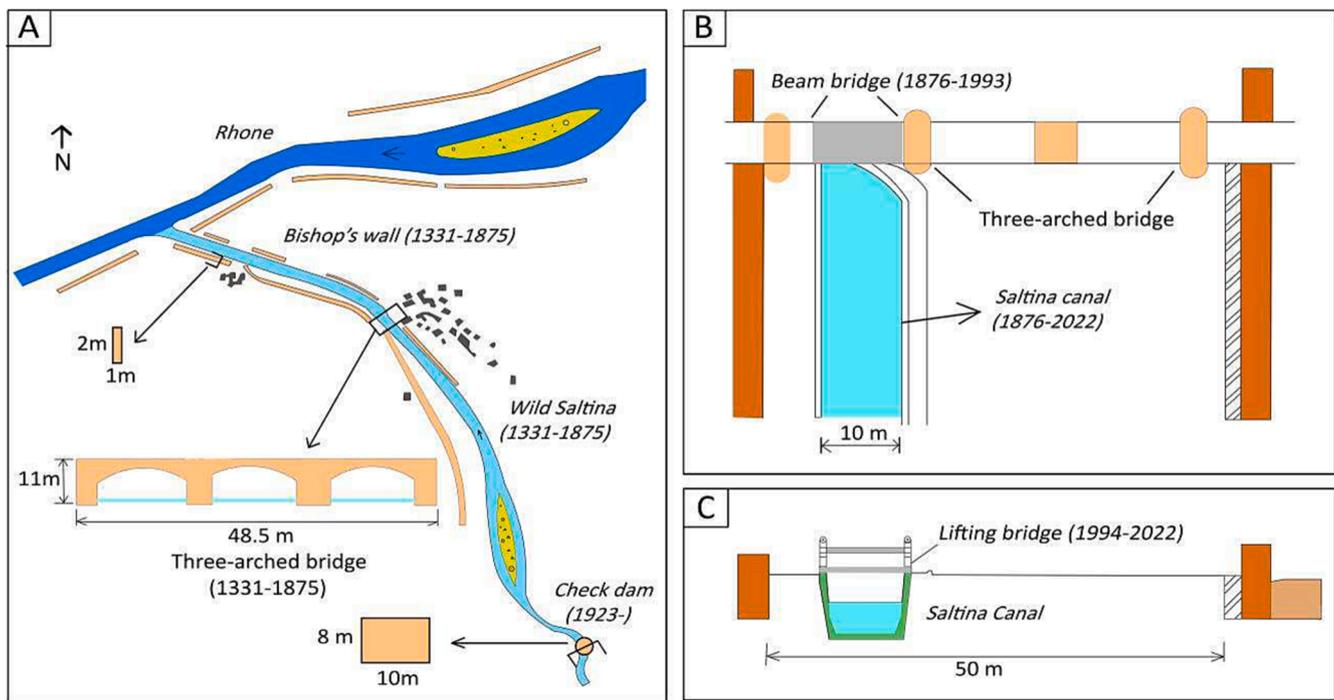
**Fig. 2.** A. Sketch of the Bishop's Wall and the three-arched bridge at the location of today's lifting bridge (inset; adapted from Meyer et al., 1997; Imboden, 1996); B. Riverbed and bankfull width area of the Saltina River above the city of Brig-Glis after 1875 (source: Imboden, 1996); C. Cross section of the "Saltina canal" and the lifting bridge.
