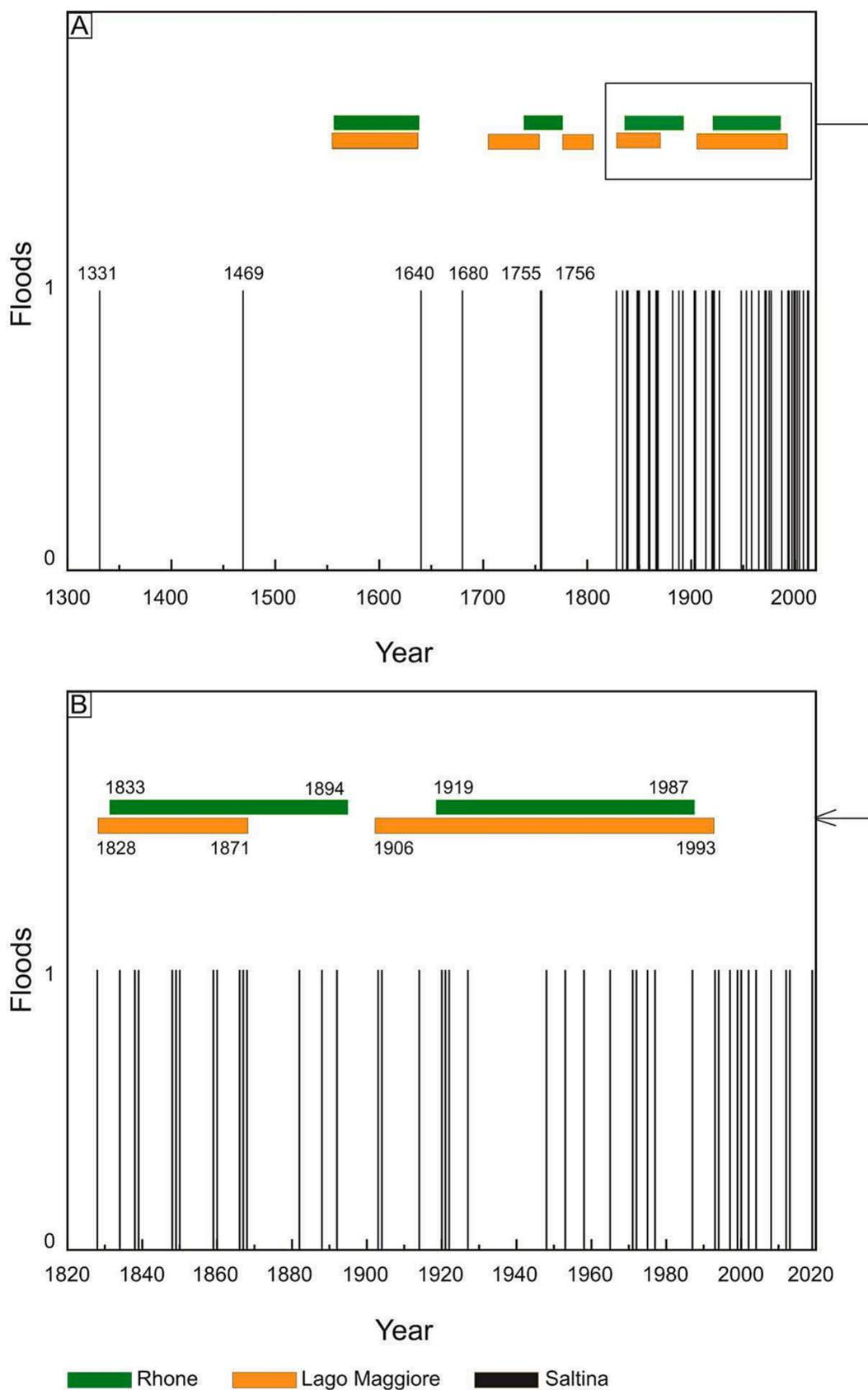
**Fig. 4.** A. Saltina flood records (1331–2020) as retrieved from historical archives and systematic gauge records compared with reconstructed floods in different larger neighboring catchments affected by comparable synoptic situations during floods. B: Detailed 1828–2020 view of flood occurrences in the Saltina River and reconstructed flood histories from the sites used in panel A.
