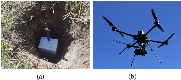
FIG. 2: a) Buried sensor node in a pasture with a limited communication range (from 20 to 250 m). b) Experimental UAV with one hour of autonomy (Tundra, Hexadrone, payload 4 kg, span 1.83 m)
