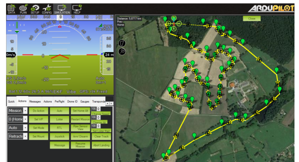
FIG. 15: The waypoints of the trajectory are reported in the mission planner of the UAV (Mission planner, ArduPilot).
