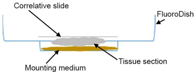
**Fig. 5** Scheme 2: Mounting of the correlative slide in a FluoroDish. Use of FluoroDishes allowing an observation of the sections between the slide and a coverslip without any damage to the sample. FluoroDishes with a high-quality glass bottom. In combination with the mounting medium, this allows to acquire excellent high-magnification images with at high resolution.
