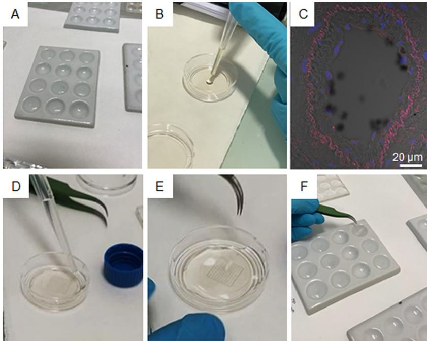
**Fig. 4** Technique for mounting and removing the correlative slide. (A) Support for immunochemistry steps. (B) End of the process and addition of Prolong Gold drop at the bottom of a FluoroDish. (C) Typical focal plane image acquired by confocal microscopy after immunolabeling, scale bar, 20  $\mu\text{m}$ . (D) FluoroDish petri filled with SPB. (E) Removal of the correlative slide. (F) Steps of dehydration.
