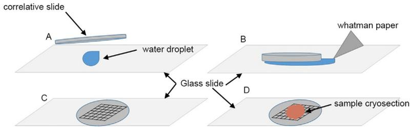
**Fig. 3** Scheme 1 for the mounting of correlative slides on glass slides. (A) Water droplet on glass slide. (B) Removal of excess water. (C) Correlative slide for use on glass slide. (D) Cryo-section on correlative slide.
