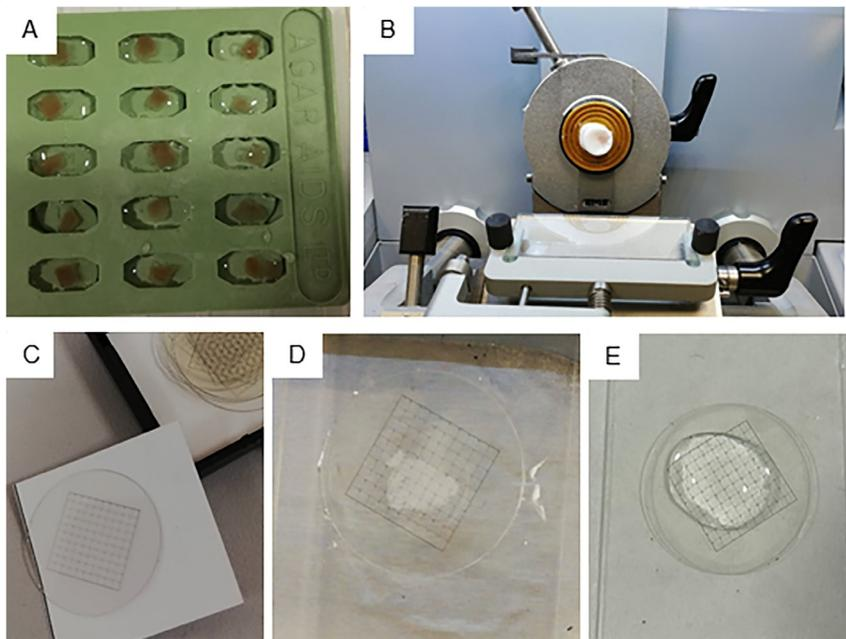
**Fig. 2** Histological workflow. (A) Mold containing samples embedding in optimal cutting temperature (OCT) medium before freezing. (B) Sectioning using a cryostat. (C) Correlative slide with graduation. (D) Section picked up on a correlative slide and positioned on a glass slide. (E) Hydration of sections before staining with toluidine blue.
