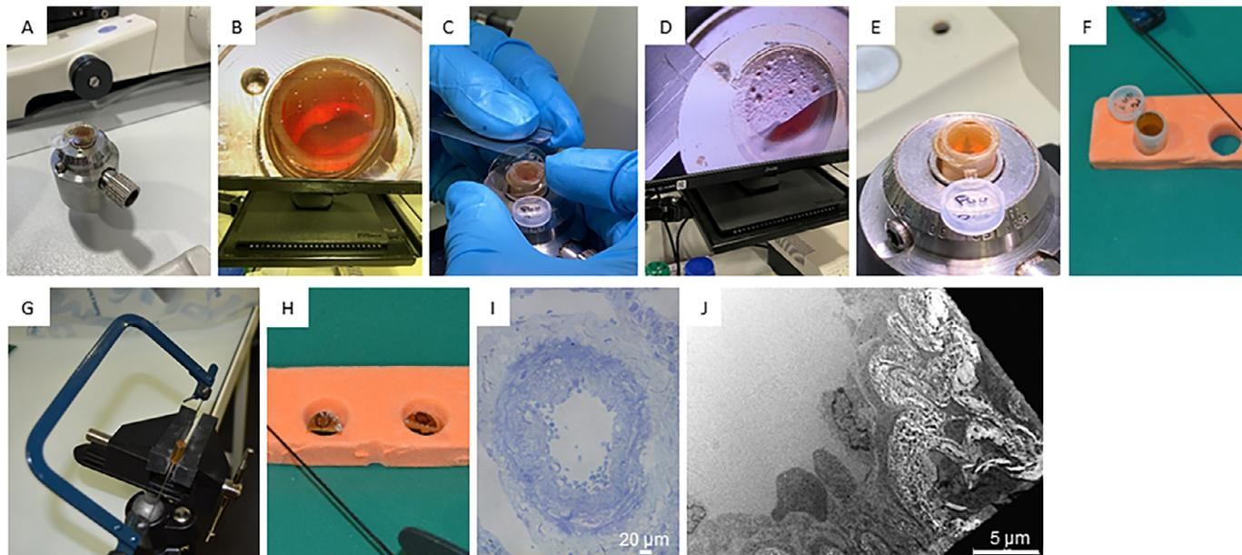
**Fig. 7** Preparation of EM blocks for ultramicrotomy. (A–D) Removal of a correlative slide from the resin block using a razor blade. (E) Tissue sample visible at the surface of the beam capsule. (F) Resin block. (G) Use of a saw to cut resin block into pieces (to increase sample size). (H) Two resin samples of the same block. (I) Semi-thick section: scale bar, 20  $\mu\text{m}$ . (J) Low-magnification TEM image: scale bar, 5  $\mu\text{m}$ .
