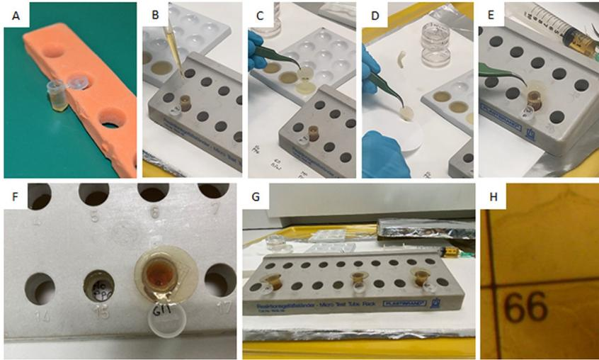
**Fig. 6** Sample preparation for electron microscopy. (A) Beam capsule almost filled (2/3) with polymerized Epon 812. (B) Filling of the beam capsule with liquid Epon 812. (C–E) Use of forceps to position a correlative slide on top of the beam capsule with the sample side facing the resin (avoiding air bubbles at this stage is crucial). (F) Correlative slide on the top of beam capsules. (G) Samples after polymerization. (H) Landmark of the correlative slide as seen on the resin block.
