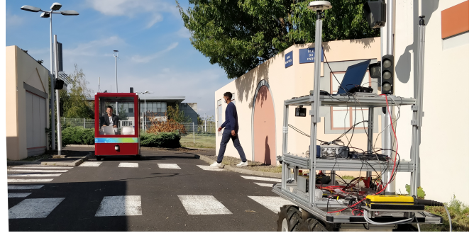
Fig. 1. Example of an urban scenario that the robot can encounter. A pedestrian is crossing the road, while a vehicle is approaching the robot in the other lane. Using the Dynamic Lambda-Fields, the robot is able to estimate the risk of its actions, taking into account a generic risk that can be adapted depending on the scenario.
