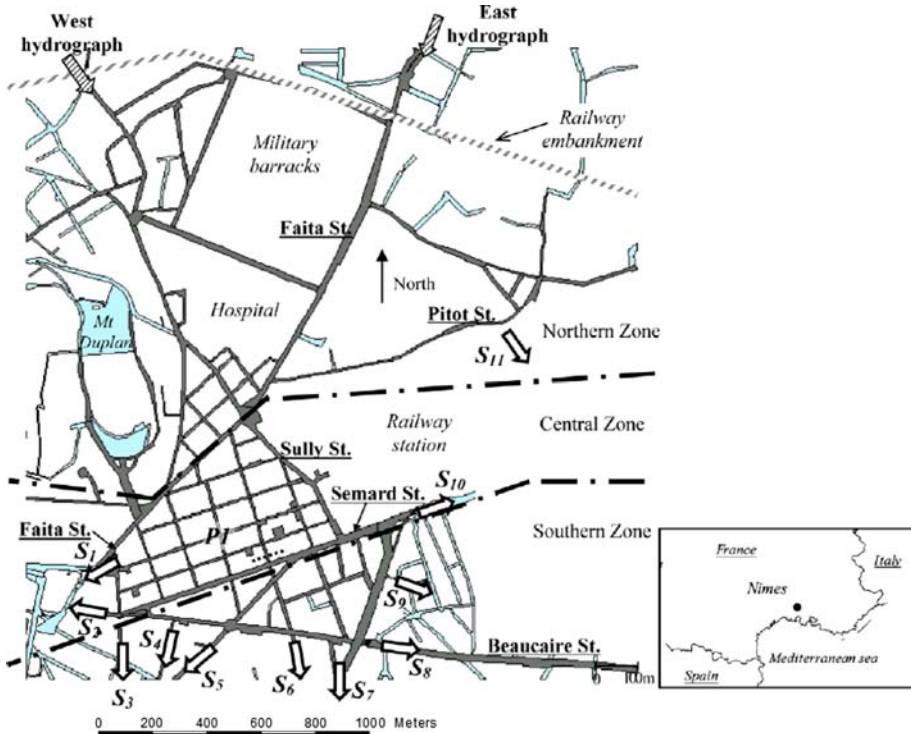
Fig. 10 The Richelieu area of the city of Nîmes for which the 1988 flood event was simulated. S1–S11 denote the outlets of the domain
