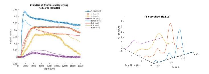
Figure 1 – Evolution of the signal profiles (left) and representative  $T_2$  relaxation time repartitions measured at the central depth (~8000  $\mu$ m; right) in function of the drying times.
