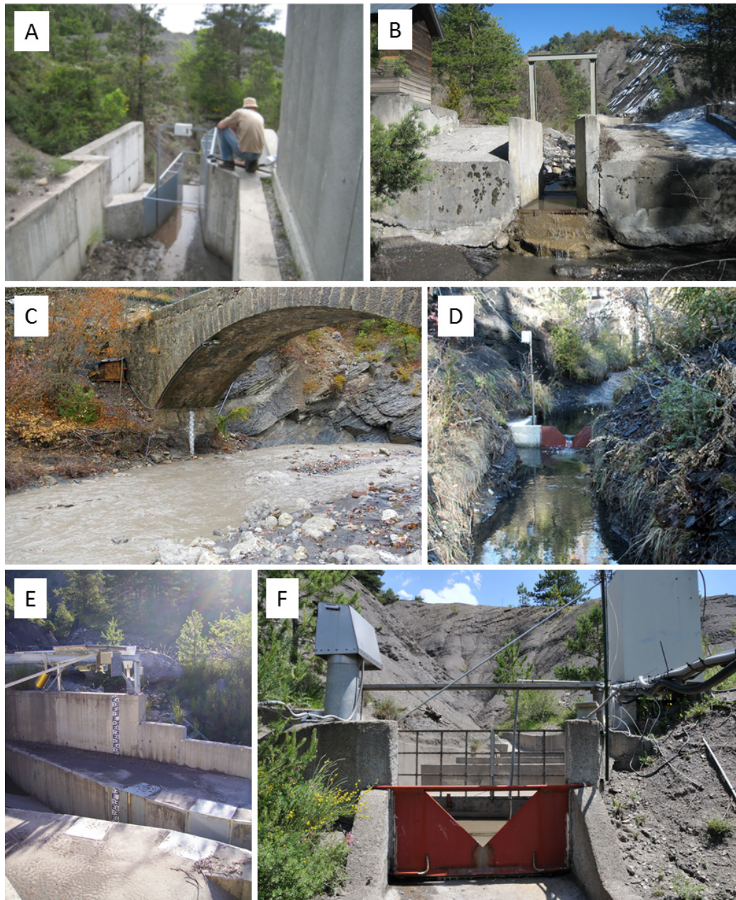
Figure 7. Photos of all the stations: (a) Moulin Parshall flume. (b) Francon Parshall flume looking upstream. (c) Bouinenc natural gauging section. (d) Brusquet low-discharge weir. (e) Laval Parshall flume. (f) Roubine weir looking upstream (photo f from Jérôme Latron).
