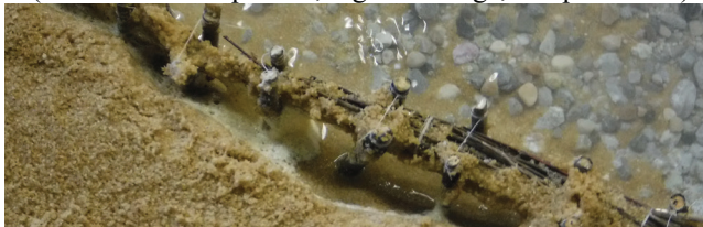
Fig.5 Top erosion (test: connection present, high discharge, full protection).
