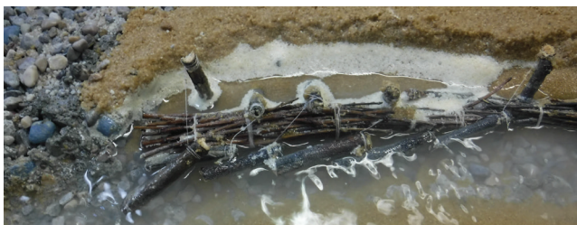
Fig. 7 Downstream back erosion (test: connection present, high discharge, no rip rap downstream).
