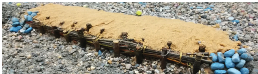
Fig.2A fascine with ripraps upstream and downstream
