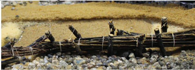
Fig.5 Top erosion (test: connection present, high discharge, full protection).
