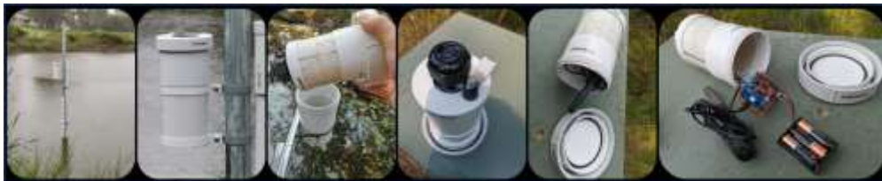
Figure 2: System installed on the field (on the left of the pole) and photos of the encapsulation system made for easy fixing and removal without changing the location of the sensor
