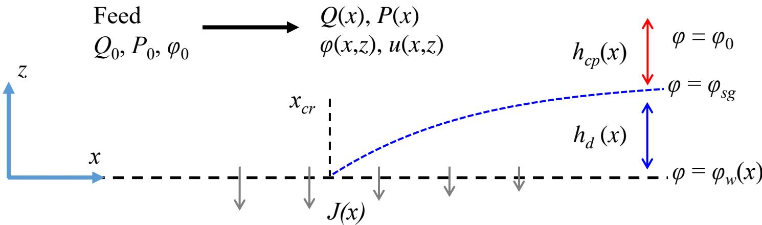
Mass balance Eq. that relates filtrate flux with solids flux in the CP layer
