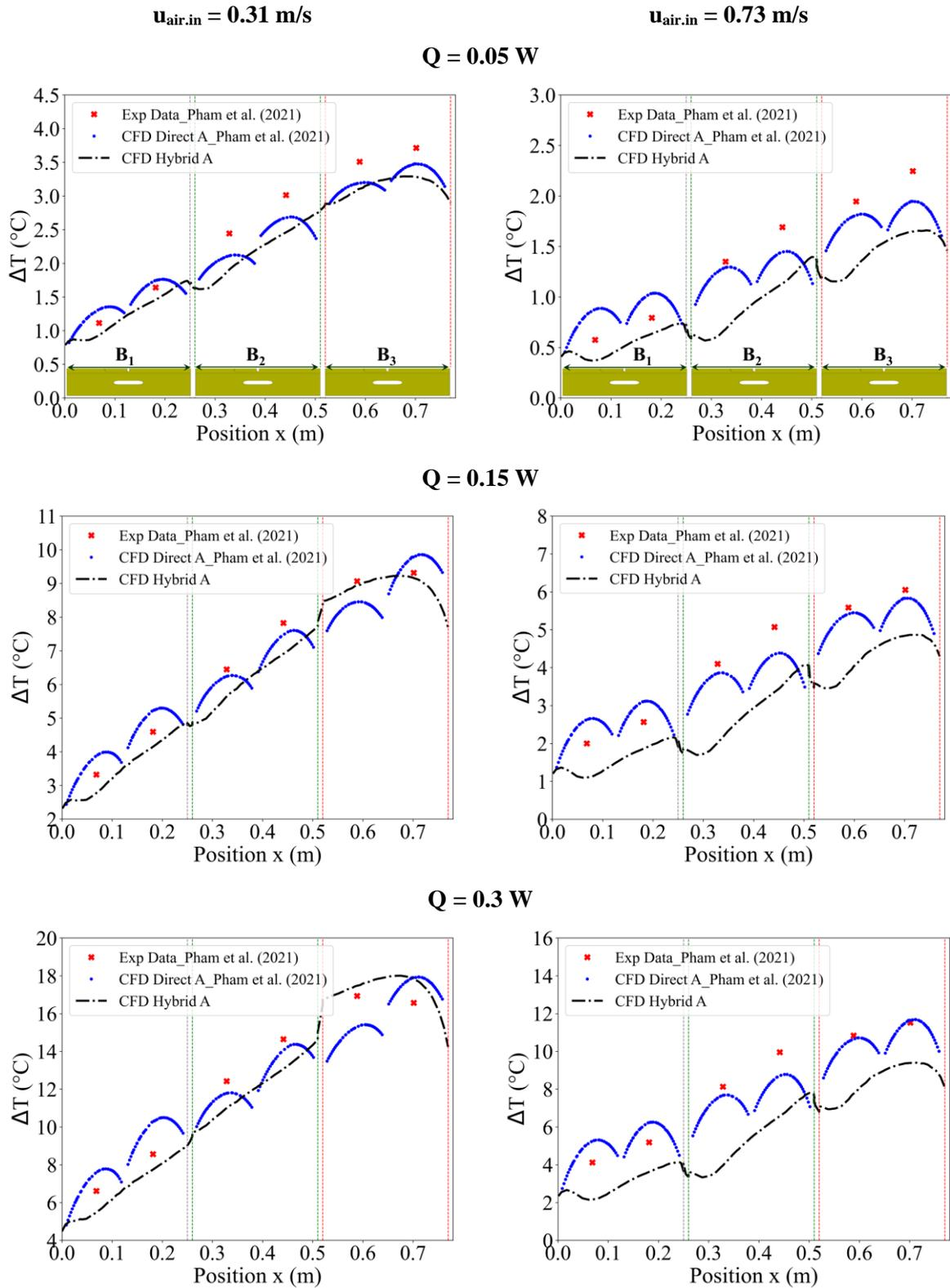
628 Fig. 6. Comparison of the temperature difference distribution ( $\Delta T = T_p - T_{\text{air.in}}$ ) obtained with the hybrid approach through the
