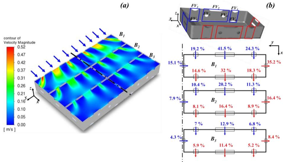
Fig. 5. Airflow distribution through the boxes for  $u_{air.in} = 0.31$  m/s and  $Q = 0W$ ; (a) air velocity magnitude at  $z = 132.5$  mm; (b) inflow and outflow rates compared to a total inflow of box  $B_1$ .
