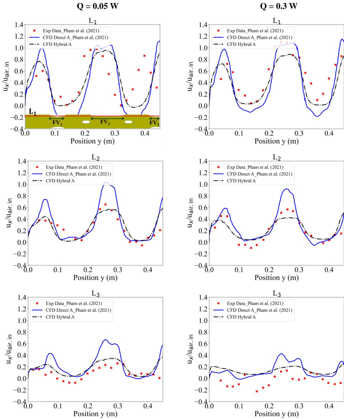
610 Fig. 4. Comparison of the air gap transversal velocity through the lines  $L_1$ ,  $L_2$  and  $L_3$  for inlet velocity 0.31 m/s and two heat
