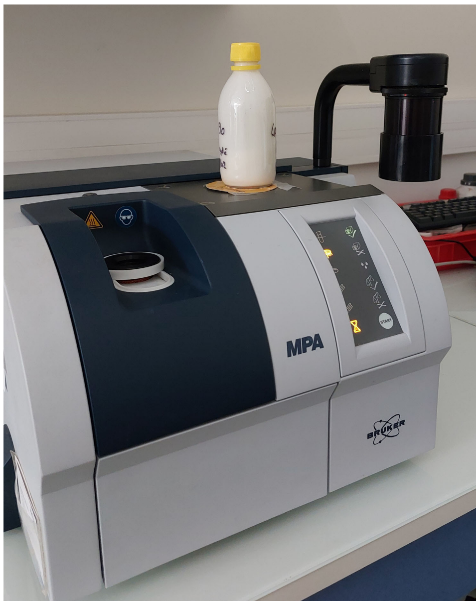
FIGURE 1 At-line analysis of emulsions by near infrared spectroscopy (NIRS) using Bruker MPA spectrometer.
