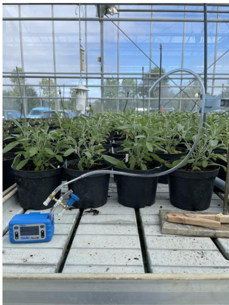
Figure 3: picture of the tool developed by ITEIPMAI. It comprises a pump and a support for capturing the volatile organic compounds (VOCs) emitted by the plants. After extraction, we obtain a volatile compound profile. This profile is then analysed as a parameter to be taken into account in the study on the impact of inter-rows in agroforestry.
