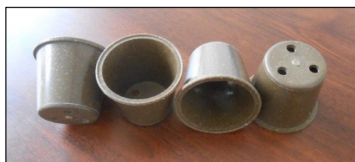
Figure 11. Example of flowerpot injected from the PHB-DFBBF-30 composite material.
