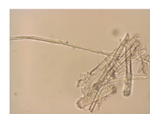
Figure 4. Optical microscope photographs of the reinforcing fibers ( \times 20 magnification).
