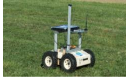
Fig. 4. Jaguar 4x4 wheel mobile robotic platform
