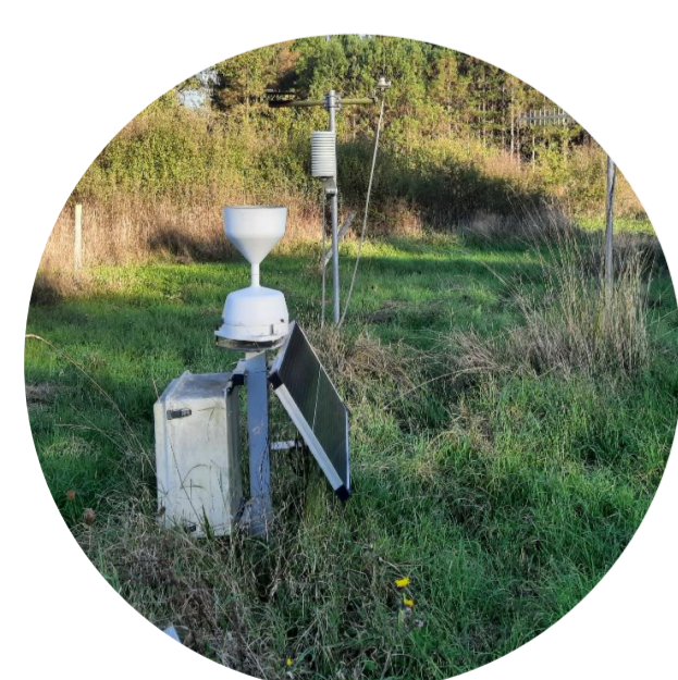
Fig 5. Weather station with hourly temperature and daily rainfall measurements
