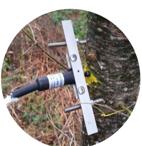
Fig 2. Automatic point dendrometer X 1 data / hour X 4 years (2020-2023) X 18 trees per SO
