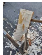
Fig. 7: hewing the surface of a shingle, photo by the author.
