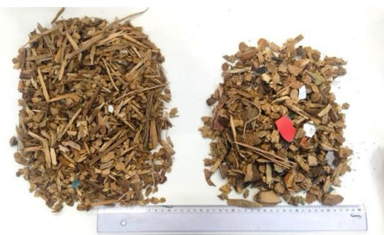
Fig. 2 :150g in the sample with a size of 6.3 mm (left) and 8 mm (right)
