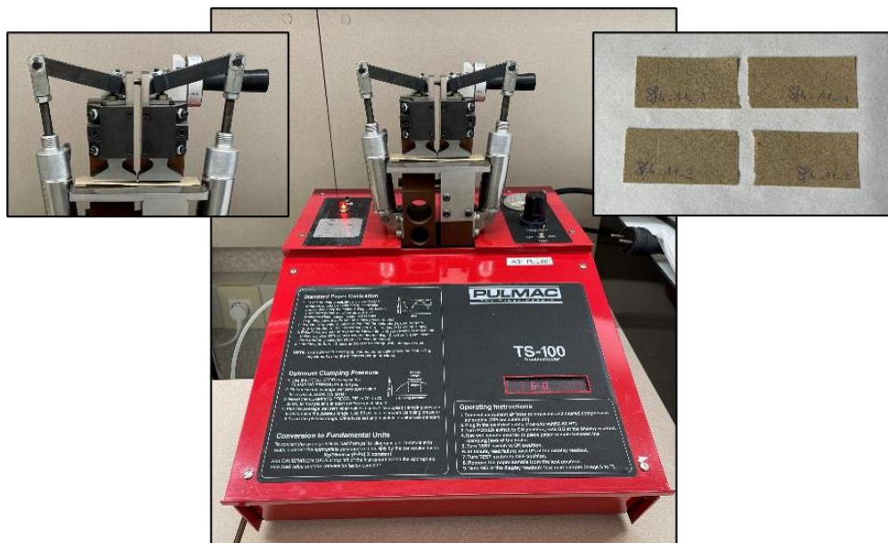
Fig. 4: Zero-span machine used for tensile tests, left: zoom of jaws containing a sample, right: samples after the test
