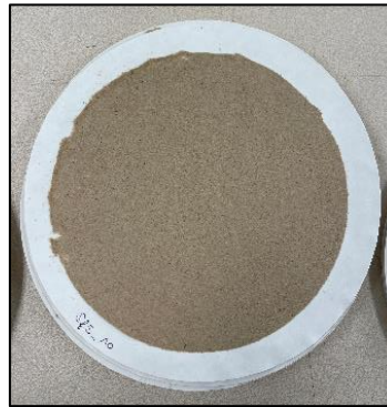
Fig. 3: Example of a 20 cm diameter handsheet containing 85% of recovered fibres and 15% of eucalyptus fibres
