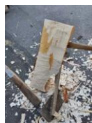
Fig. 7: hewing the surface of a shingle, photo by the author.
