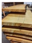
Fig. 9: pith crack on the top end of a twenty-two millimetres board, photo by the author.
