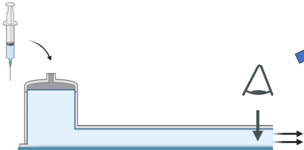
Unidirectional drying cell
