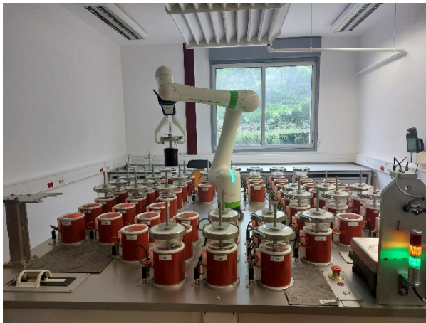
Figure 4. Vinimag : Automated fermentation system.
