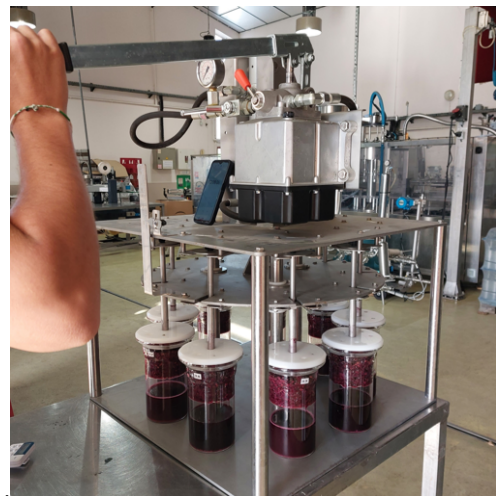
Figure 6. Nano'Press : 9-station pressing system.
