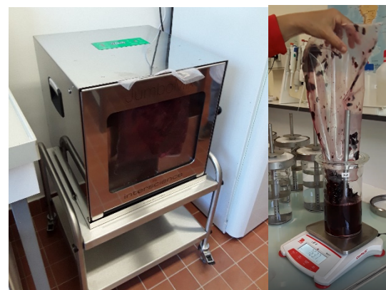
Figure 2. Grapes kneaded in a bag (left) then transferred to a fermenter (right).
