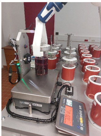
Figure 5. Vinimag measuring station: weighing and colour.
