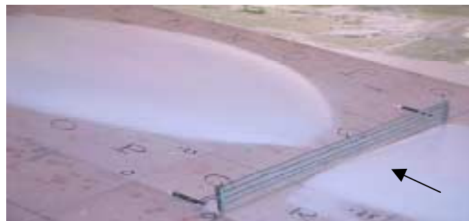
Figure 12: Porous snow fence on a 10° slope after 8 minutes.
