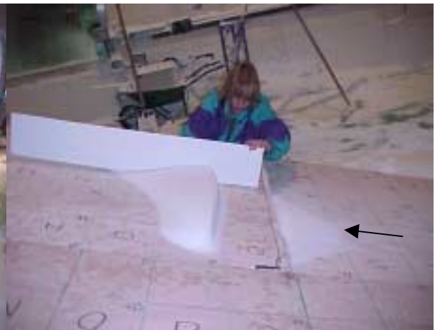
Figure 10: Determination of snowdrift shape at the end of an experiment
