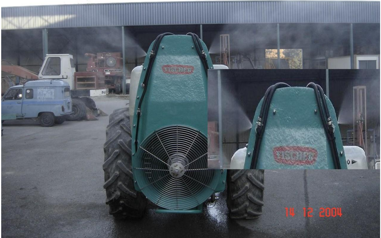
FIG. 4.9 – Air-assisted sprayer and nozzle output.
