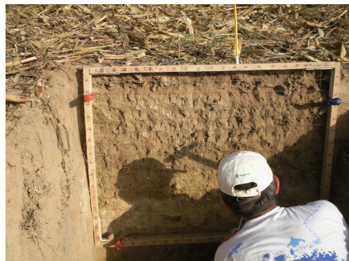
Fig. 3. Experimental study of the profile of maize roots using a soil pit. The vertical plane that is perpendicular to the maize rows is divided to square cells (5×5 cm). A note from 0 to 5 is assigned to each cell by observing the presence of roots in a soil layer of 1 cm thick.
