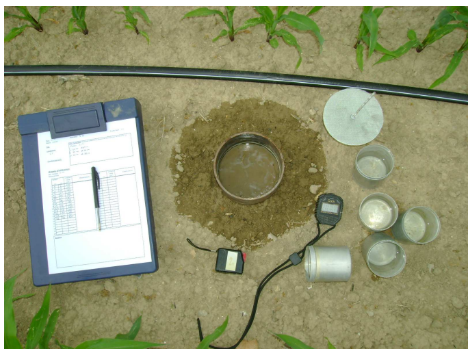
Fig 1. Beerkan infiltration method: known volumes of water are successively infiltrated and the time passed during each infiltration is recorded.
