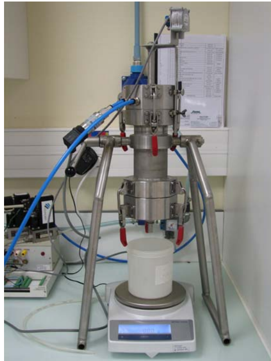
Figure II. 13 : La Cellule de Filtration-Compression
