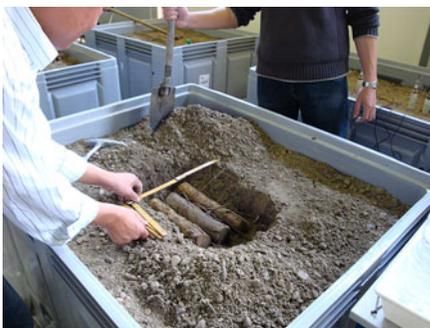
**Fig. 5** Three ash samples in longitudinal orientation
