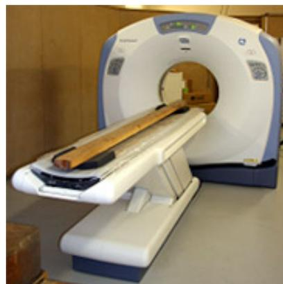
**Photo II.21 : Scanner Medical General Electric Brightspeed Exel (INRA).**
