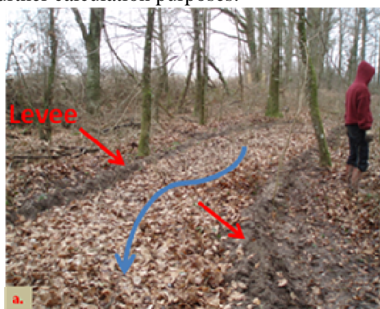
Fig. III-15: Experimental plot; (a) levees (red arrows) and runoff direction (blue arrow); (b) outlet flow constriction (water color is due to injected uranine). From (Richard, 2009).
