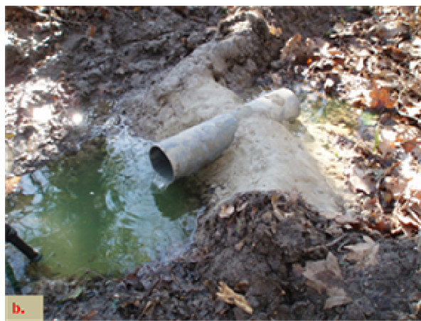
Fig. III-15: Experimental plot; (a) levees (red arrows) and runoff direction (blue arrow); (b) outlet flow constriction (water color is due to injected uranine). From (Richard, 2009).
