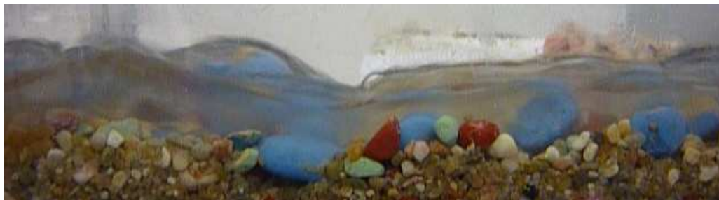
Figure 11 : Shallow flow over a non uniform grain size distribution in a flume
