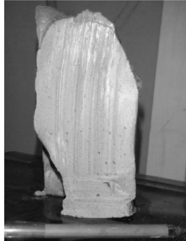
465 Fig. 9: Slice of consolidated FFT (top corresponds to anode location and bottom to cathode).
