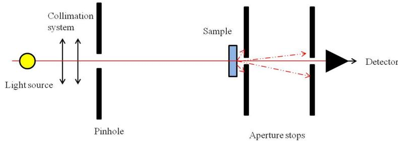
Figure 1.4: Experimental setup for regular transmittance measurements.
