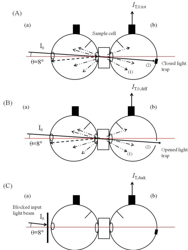
Figure 1.22: (A) Experimental measurement of the input totally transmitted  $I_{T,0,tot}$  signal. (B) Experimental measurement of the input diffusely transmitted light  $I_{T,0,diff}$ . (C) Experimental measurement of the dark signal  $I_{T,dark}$  in the transmittance sphere.
