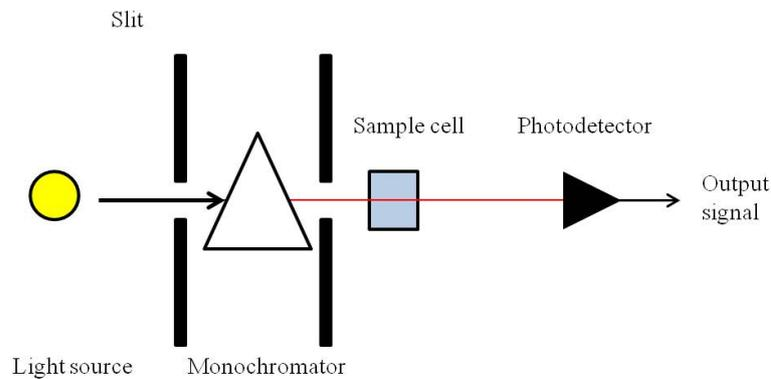
Figure 1.7: Schematic of the single-beam spectrophotometer configuration.
