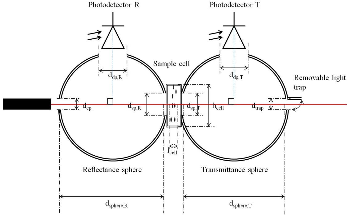
Figure 1.12: Side view of the double integrating sphere setup
