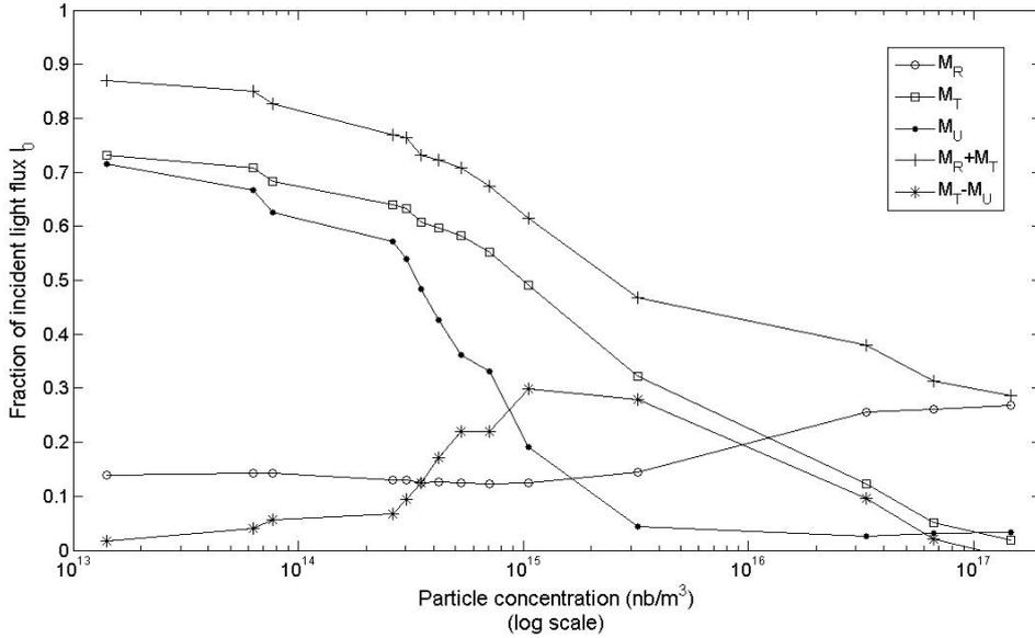
Figure 1.24: Fraction of the incident light  $I_0$  respectively reflected ( $M_R$ ), transmitted ( $M_T$ ) and regularly transmitted ( $M_U$ ) by the samples put in a 5mm-sample cell, as a function of the particle concentration. The quantity  $M_R + M_T$  expresses the total fraction of  $I_0$  that was measured with the DIS setup.  $M_T - M_U$  is the fraction of  $I_0$  that was diffusely transmitted by the sample
