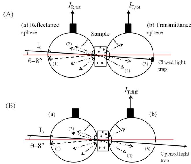
Figure 1.21: (A) Experimental measurements of the totally reflected  $I_{R,tot}$  and totally transmitted  $I_{T,tot}$  signals. (B) Experimental measurement of the diffusely transmitted light  $I_{T,diff}$ .
