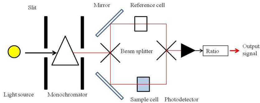
Figure 1.6: Schematic of the dual-beam spectrophotometer configuration.
