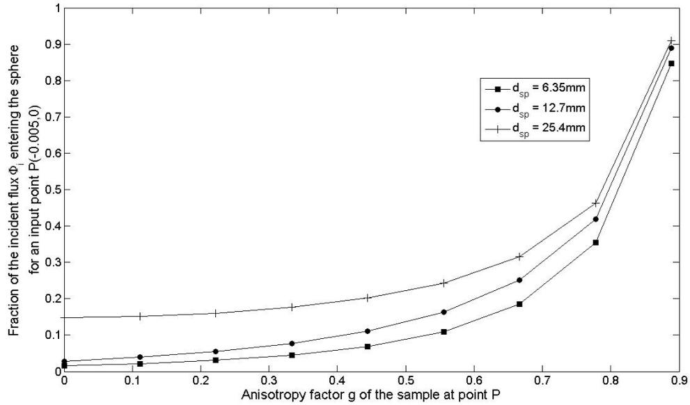
Figure 1.18: Fraction of the incident flux  $\Phi_i$  on the point  $P(-0.005, 0)$  on the sample actually entering the sphere for various values of the sample port diameter  $d_{sp}$  and various anisotropy factor  $g$
