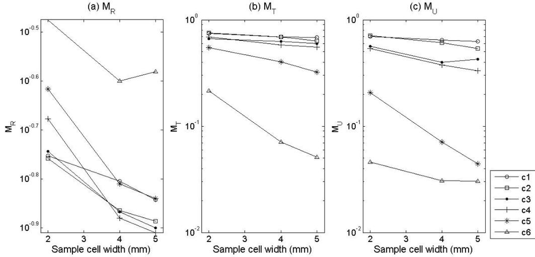
Figure 1.25: (a) Reflected ( $M_R$ ), (b) transmitted ( $M_T$ ) and (c) regularly transmitted ( $M_U$ ) light measured at different particle concentrations for the three sample cell size, namely 2mm, 4mm and 5mm wide. The particle concentrations are expressed in particles/ $m^3$  such that  $c_1 = 7, 7.10^{13}$ ,  $c_2 = 3.10^{14}$ ,  $c_3 = 4, 2.10^{14}$ ,  $c_4 = 7.10^{14}$ ,  $c_5 = 3, 2.10^{15}$ ,  $c_6 = 6, 6.10^{16}$ .
