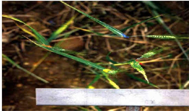
FIGURE 2.16: In-field reflectance correction using a calibrated ceramic plate.
