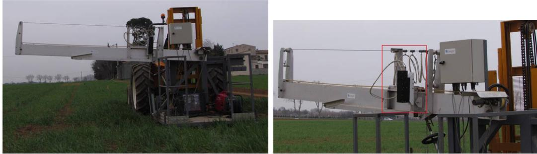
FIGURE 4.2: Illustration of Irstea acquisition setup for in-field measurements. The Hypsux camera is in the red rectangle on the right figure.
