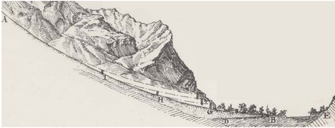
Figure 1.1 – Retention check dam optimal location (at point G) to promote retention in gorges (after Breton, 1867)
