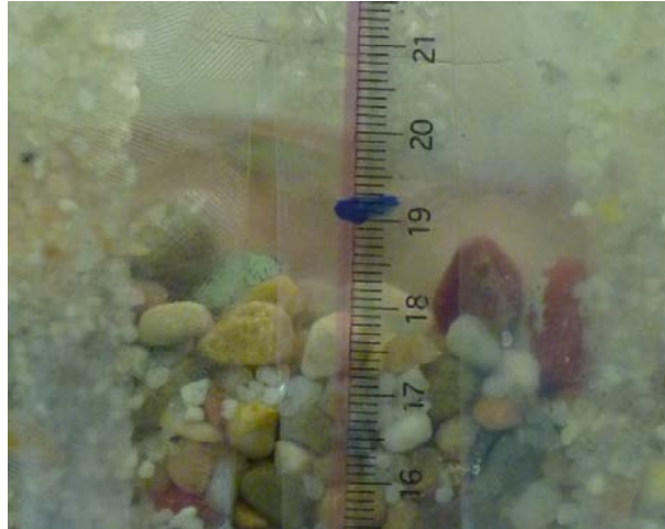
Figure 5.20 – Picture of a bed level measurement window with the transparent staff gauge. The coarse material of the bed was the biggest source of uncertainties. Here, for instance, the bed level would have been estimated as 18.1 \pm 2 \text{ mm}
