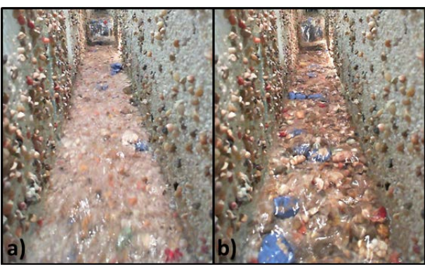
Figure 5.5 – Rough flume side walls and bed states at the same position at different time: a) fine bed during a bed-load sheet event, b) paved bed with high grain protrusion, 3'30'' later
