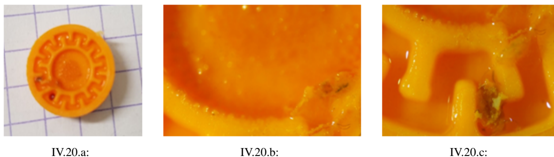
Figure IV.20: Global view of the dripper with a diamond marker shapes (a), presence of whitish granular fouling in the central zone (b), residue at the 1 st baffle (c).
