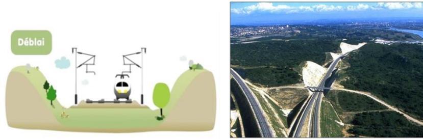
FIGURE I-29: DEBLAI SCHEMA ET PHOTO
