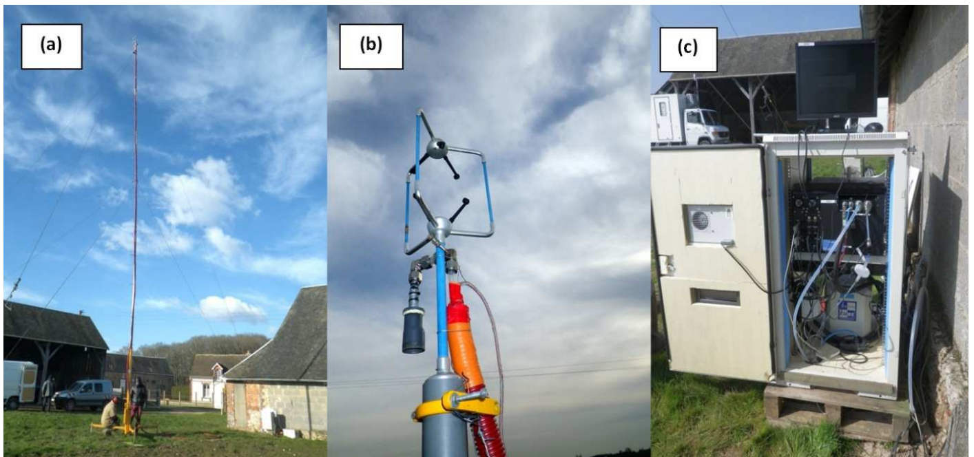
Figure 33: (a) The 15 meters mast, (b) The anemometer at the top of the mast and the inlet of gas, (c) the quantum cascade laser spectrometer to measure N 2 O concentration
