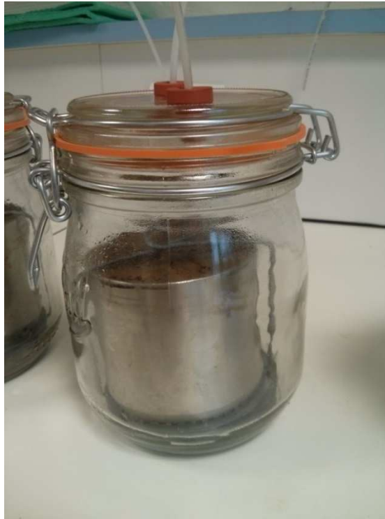
Figure 20: Cylinder of soil placed into a glass jars with inlet and outlet tube on the top.
