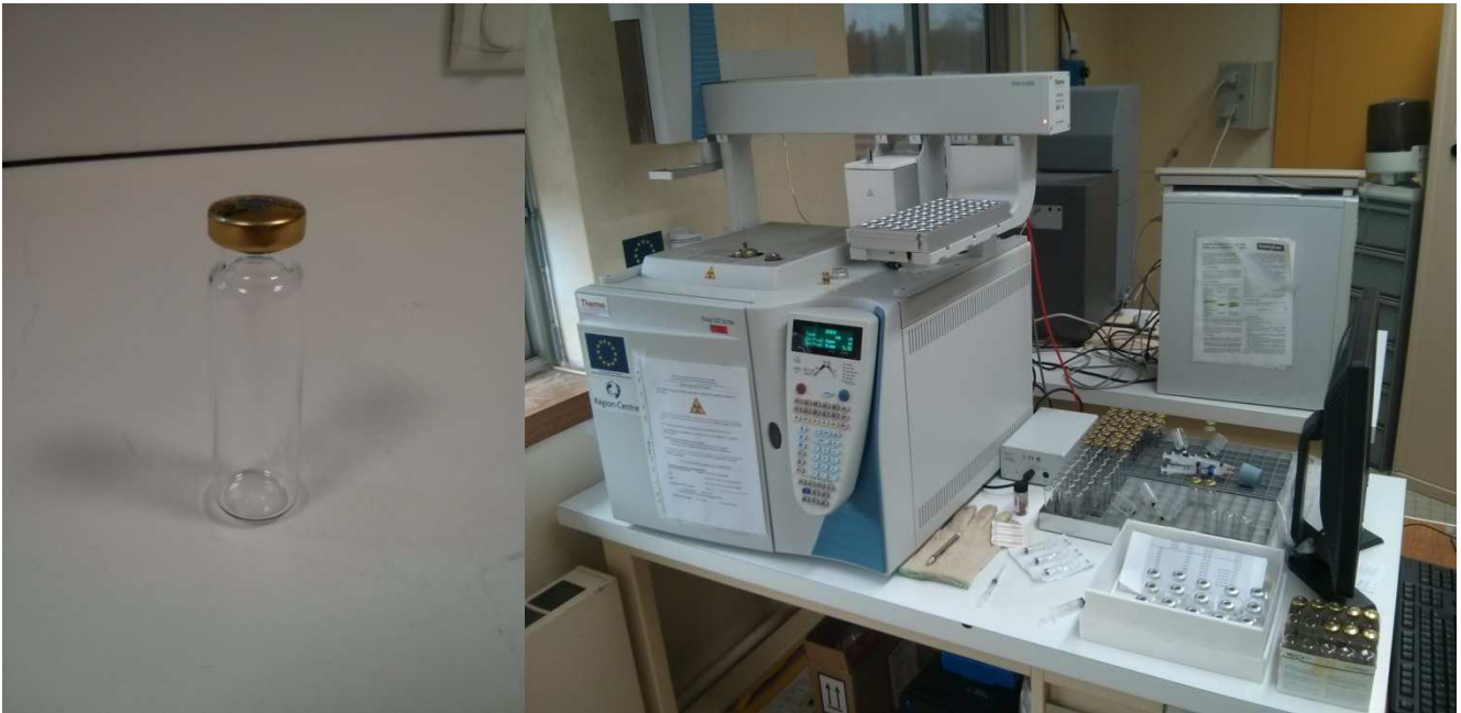
Figure 23: Photo of a vacuumed vial used for gas sampling and the gas chromatograph where gases were analyzed.
