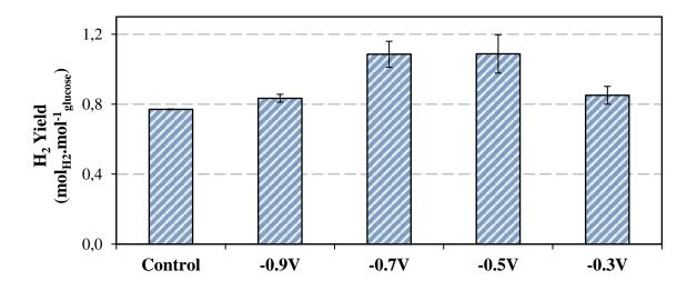
Fig. 3-6: Hydrogen yield observed during electro-fermentation tests at different potential applied on the working electrode using single chamber reactors
