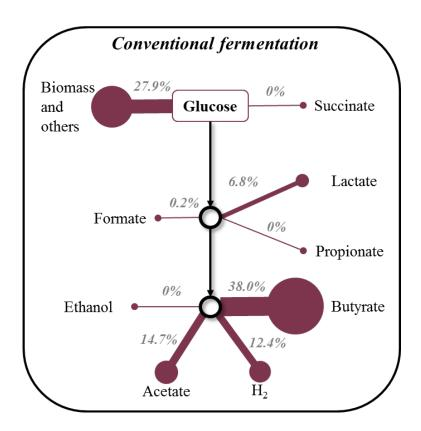
Fig. 5-2: Metabolite distribution observed during steady state of continuous operation when conventional fermentation (CF) was performed
