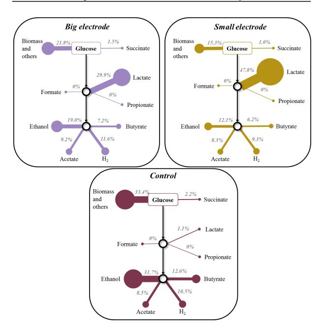
Fig. 3-11: Metabolite distribution observed during electro-fermentation tests comparing two electrodes sizes using dual-chamber reactors
