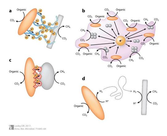
Fig. 1-8: Proposed mechanisms for interspecies electron transfer through Direct interspecies electron transfer (DIET)
