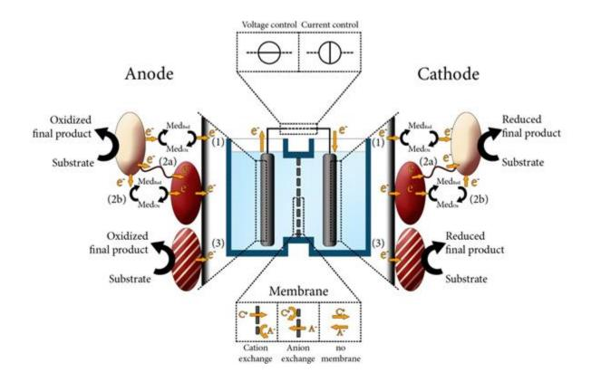
Fig. 1-6: Process configurations of electro-fermentation system including possible interactions between electrode and fermentation medium
