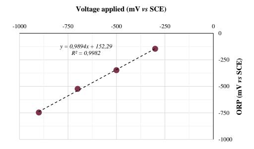
Fig. 3-9: Linear correlation between ORP measured in fermentation bulk and potential applied at working electrode
