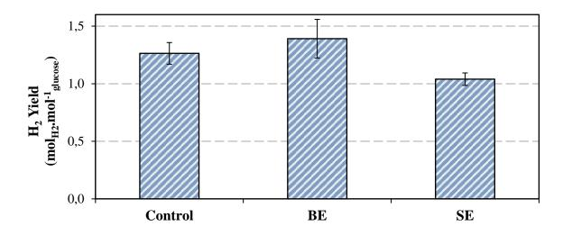
Fig. 3-10: Hydrogen yield observed during electro-fermentation tests comparing two electrodes sizes using dual chamber reactors
