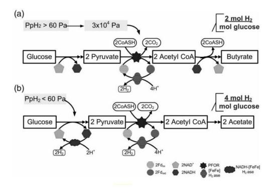
Fig. 1-3: H<sub>2</sub> partial pressure effect on dark fermentation pathway
