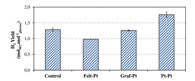
Fig. 3-1: Hydrogen yield observed during Electro-fermentation tests using single chamber reactors and different electrode materials
