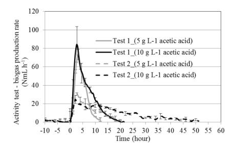
Figure 35: Activity test: biogas production rate after injection of leachate containing acetic acid.  $1^{st}$  injection is effectuated after the methane peak (after about 30 days) and  $2^{nd}$  injection at the end of digestion (after about 80 days). Two acetic acid concentrations in the leachate were tested: 5 g  $L^{-1}$  and 10 g  $L^{-1}$ .
