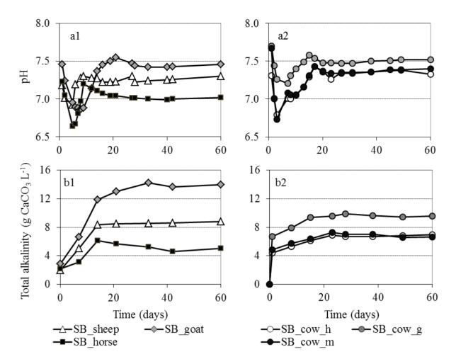
Figure 11: Parameters monitored in the leachate during the digestion process in a LBR of six different spent animal bedding: (a1 - a2) pH and (b1 - b2) total alkalinity in g CaCO<sub>3</sub> L<sup>-1</sup>
