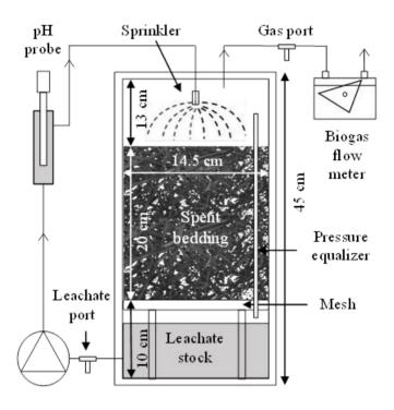
Figure 19: Experimental leach-bed reactor (LBR)
