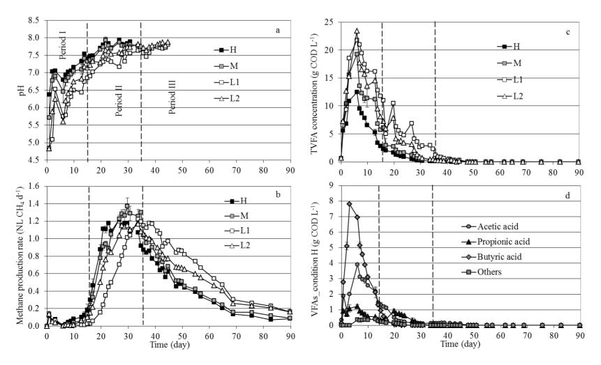
Figure 34: Parameters measured during the digestion process: (a) pH; (b) methane production rate; (c) total volatile fatty acids (TVFA) concentration; (d) volatile fatty acids (VFAs) concentration (condition H). H and M refers to the mean value of H1- H2 and M1 - M2, respectively, during period I and period II while, they correspond to only H1 and M1, respectively, during period II
