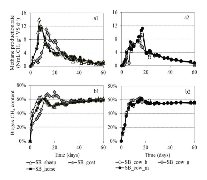
Figure 13: (a1 - a2) methane production rate in NmL CH<sub>4</sub> g<sup>-1</sup> VS d<sup>-1</sup> and (b1 - b2) methane content in biogas during the digestion process of six different spent animal bedding in a LBR
