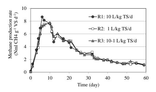
Figure 16: Methane production rates of three LBRs with different internal recirculation conditions
