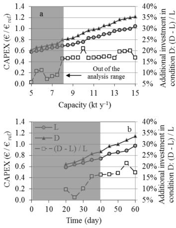
Figure 23: Results of the economic simulation performed on an industrial site using a sequential LBR process considering a digester number varying from 4 to 9 and an electric cogeneration power ranging from 100 to 300 kW $_{\rm el}$ . Evolution of the CAPEX in relation to (a) the annual capacity and (b) the batch duration
