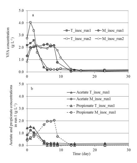
Figure 27: Comparison of mesophilic ( $M_{inoc}$ ) and thermophilic ( $T_{inoc}$ ) conditions: (a) VFA concentration in run 1 and run 2; (b) acetate and propionate concentrations in run 1
