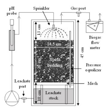
Figure 10: Experimental leach-bed reactor
