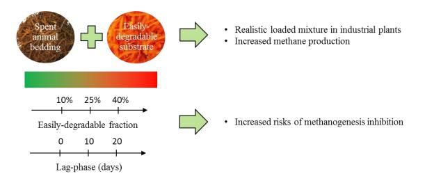
Figure 41: Effect of the addition of a fraction of easily-degradable substrate to spent animal bedding
