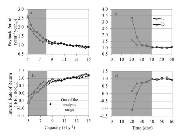
Figure 22: Results of the economic simulation performed on an industrial site using a sequential LBR process considering a digester number varying from 4 to 9 and an electric cogeneration power ranging from 100 to 300 kW $_{\rm el}$ . Evolution of the (a) Payback Period and Internal (b) Rate of Return in relation to the annual capacity. Evolution of the (c) Payback Period and (d) Internal Rate of Return in relation to the batch duration
