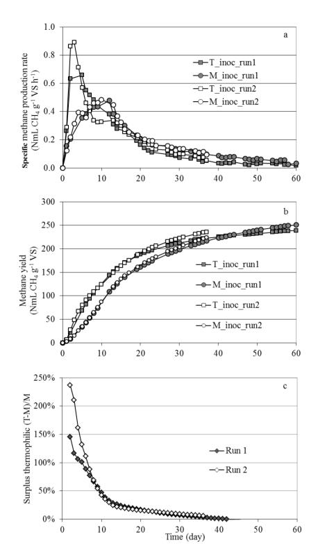
Figure 26: Comparison of mesophilic ( $M_{inoc}$ ) and thermophilic ( $T_{inoc}$ ) conditions, in run 1 and run 2: (a) specific methane production rate; (b) methane yield; (c) additional methane yield in thermophilic conditions
