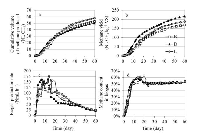
Figure 20: Comparison of the biogas parameters analysed all along the digestion process of three different experimental loadings: spent cow bedding and water (B), spent cow bedding and leachate (L) and spent cow bedding and digestate (D). (a) cumulative methane produced, (b) methane yield, (c) biogas production rate and (d) methane content in biogas produced; (b) methane yield; (c) biogas production rate; (d) methane concentration in biogas
