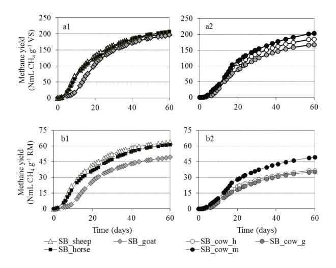
Figure 14: (a1 - a2) methane yield in NmL CH<sub>4</sub> g<sup>-1</sup> VS, (b1 - b2) methane yield in NmL CH<sub>4</sub> g<sup>-1</sup> RM (raw mass) during the digestion process of six different spent animal bedding in LBRs
