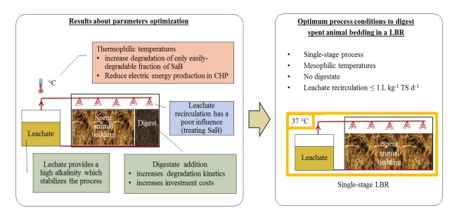
Figure 40: Results of the parameters optimization and optimum process conditions to digest spent animal bedding in a LBR
