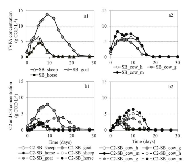
Figure 12: Volatile fatty acids measured in the leachate during the digestion process in a LBR of six different spent animal bedding: (a1 - a2) total volatile fatty acids concentration in g COD L<sup>-1</sup>, (b1 - b2) acetic (C2) and propionic (C3) acid concentrations in g COD L<sup>-1</sup>
