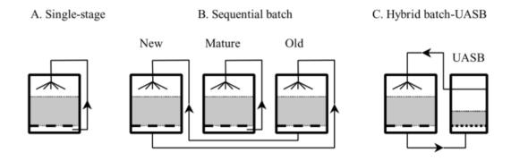
Figure 2: Existing LBR configurations (Vandevivere et al., 2003)
