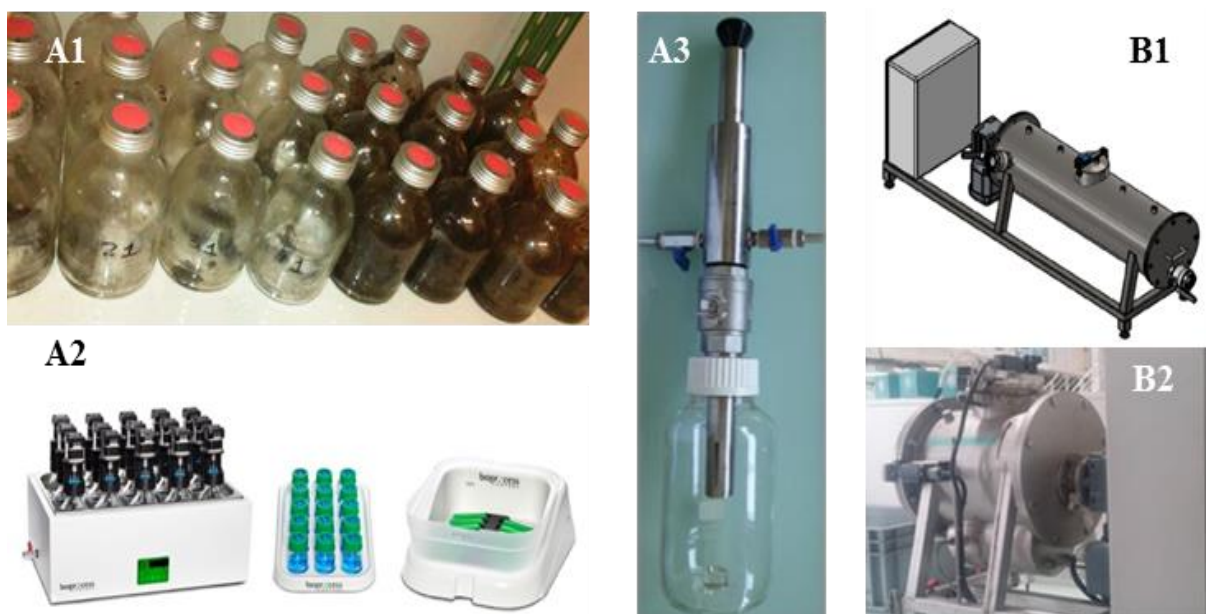
Figure 2.2. Pictures and schemes of the different reactors used during the thesis: (A1) discontinuous laboratory-scale reactors, (A2) AMPTSII system, (A3) discontinuous dry AD reactors and (B1 and B2) pilot-scale reactors
