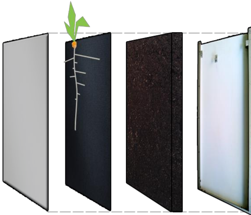
Figure II-10 Illustration of the rhizotron device used for the observation of maize root systems. Root systems are allowed to develop in a plane between a transparent plexiglass layer placed at the front and a nylon fabric preventing the roots from entering into the substrate. Different layers are (from left to right): 5 mm thick plexiglass plate, nylon fabric, 2 cm layer of substrate, 5 mm thick extruded polystyrene plate.
