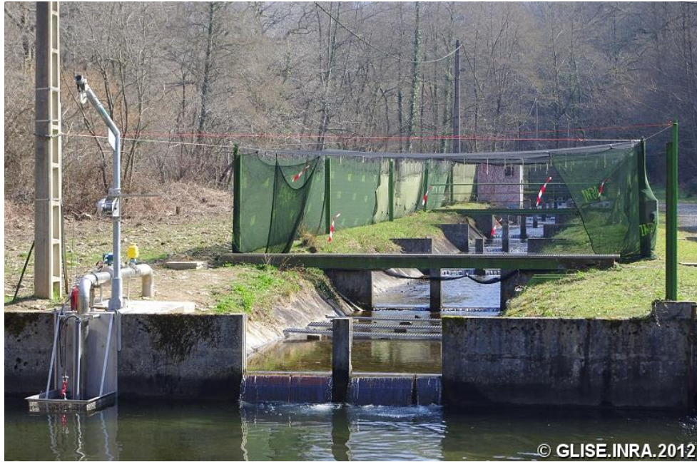
Figure 1. Lapituxuri experimental channel. Nets are deployed to prevent birds from fishing. Passage between sections can be prevented if required. Substratum can be modified, as well as water depth and shelters availability. Additionally, water discharge can be controlled by tuning the in-flow from the natural river, independently for sections 2 to 7 and 8 to 13 respectively (thanks to a by-pass) and can also be regulated using a water pump (lower left corner of the picture).
