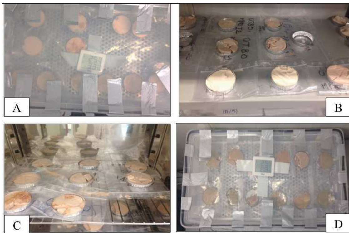
Figure 7. Pictures of the climatic chambers: A=33% RH at 25°C; B=60% RH at 25°C; C=75% RH at 25°C; D=90% RH at 25°C
