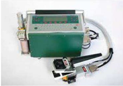
Figure 10: LICOR© LI-6400XT pro (LiCor©, Lincoln, Neb. USA).
