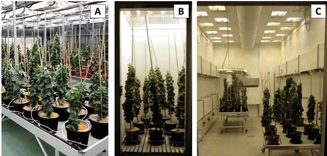
Figure 10: Experimental devices. Microvine plants grown in greenhouse (A), 1 m 2 growth chamber (B) and 20m 2 growth rooms (C).
