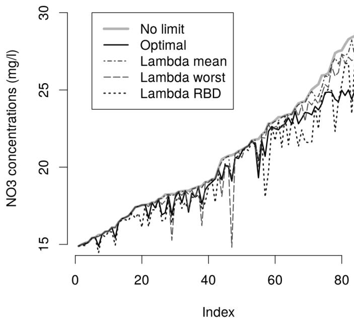
(a) Reference NO<sub>3</sub> concentrations (livestock variation and no environmental constraint) and the resulting concentrations from the application of the four scenarios, namely the optimal adjustment and the taxation with average, maximal and aggregated  $\lambda_w$  values. The x-axis is giving the index of the sectors in ascending order following the reference NO<sub>3</sub> concentrations.
