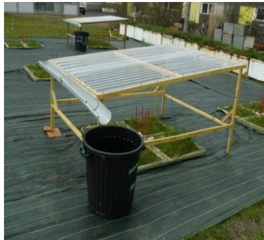
Figure 3-2 Rainfall shelter equipped with gutters and a water butt.
